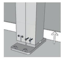
4. Drill six ø5.5 mm holes after the section is installed level
