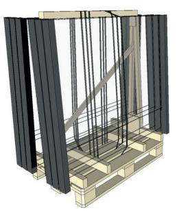
Loosen the straps gradually as sections are installed. Each package can hold up to 6 sections.
